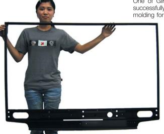
One of GIHKs customers has recently successfully applied internal gas assisted molding for production of a 57" LCD TV
